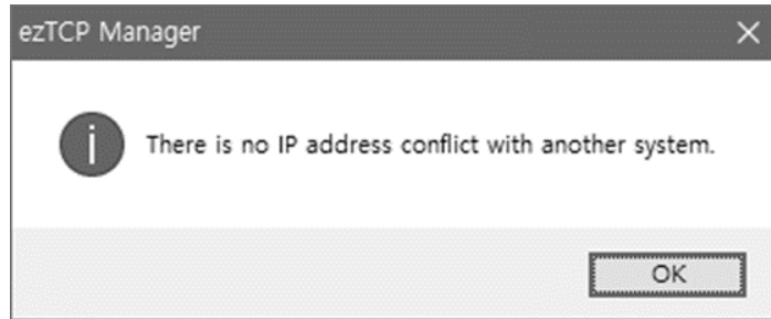
Figure 7-13 Without IP address conflict detection
