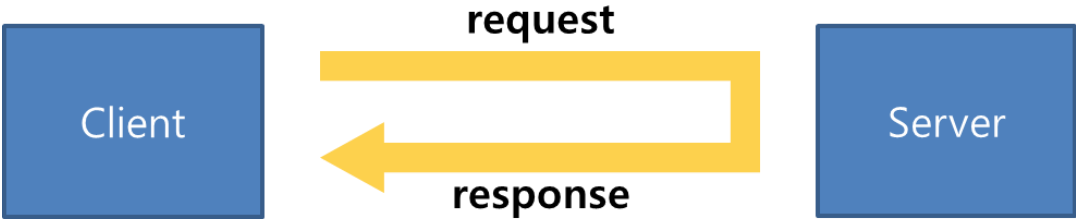
Figure 3-3 MODBUS Client/Server Model
