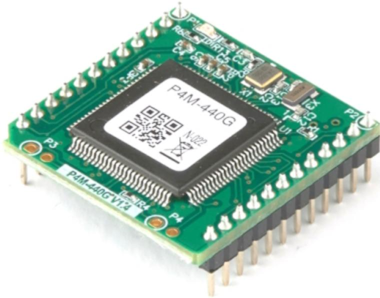
P4M-440G is an MQTT client module. This module accepts AT commands via the UART port, providing various features for MQTT communication. As a result, users can implement MQTT functionality on their MCU (Microcontroller) or microcomputer using this module.
