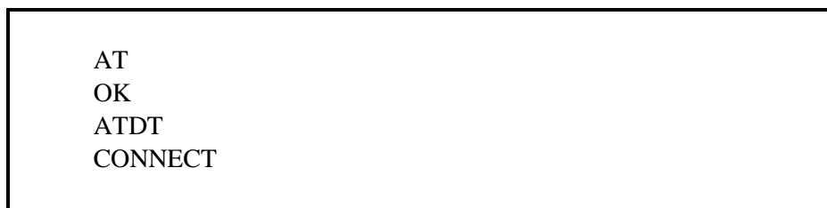
Figure 3-2 Example of dialing with CDMA modem
