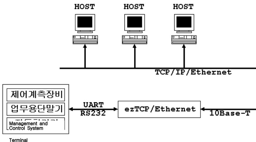
If an OA instrument (hereafter a host) is connected to the TCP port of ezTCP over an Ethernet network, the serial port of the DTE is connected virtually to the TCP port of the host. Then, ezTCP will function as an intermediate device between the serial port and the TCP port.
