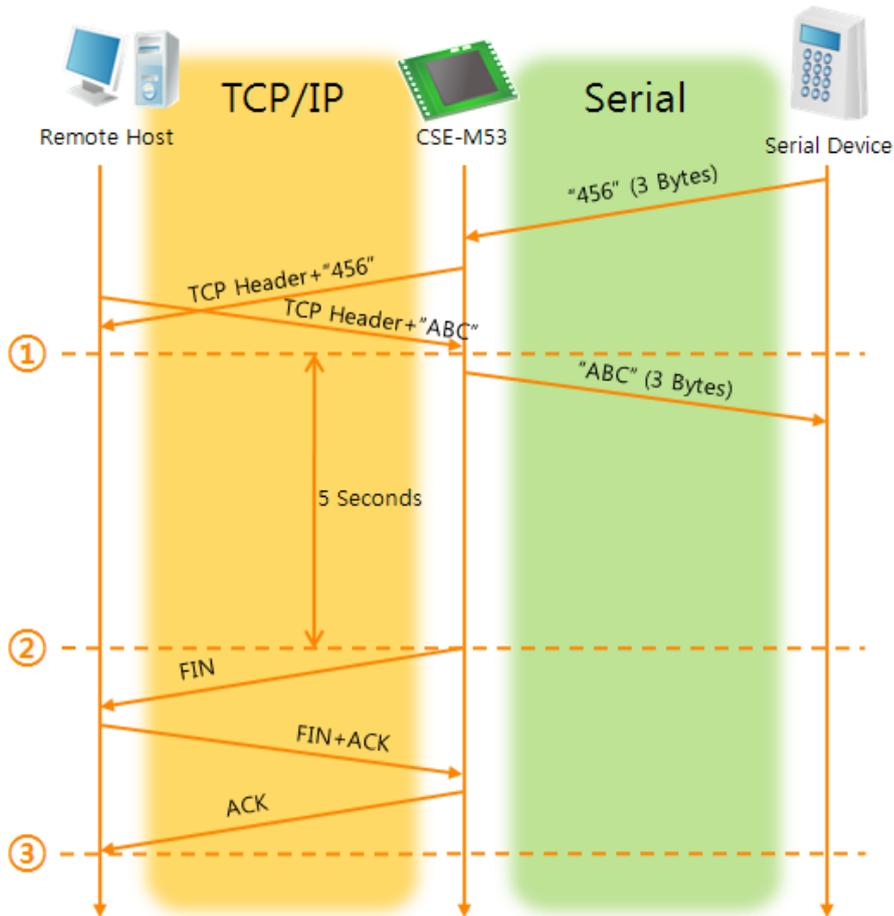
Figure 5-3 time chart for a situation that [Timeout] is set to 5
