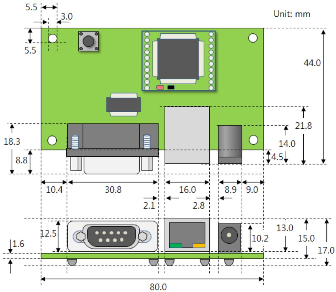
Figure 1-6 Dimension of evaluation board
