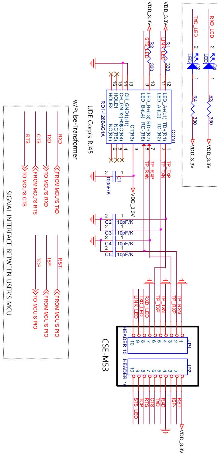
Fig 1-1 an Application Circuit
