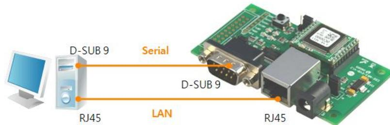
Figure 2-1 connection between CSE-M53 and a PC
