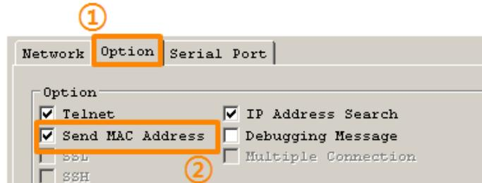
Figure 7-2 setting of Sending MAC Address function
