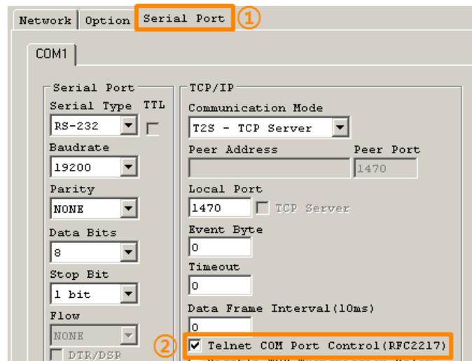
Figure 7-3 setting of TELNET COM Port Control option
