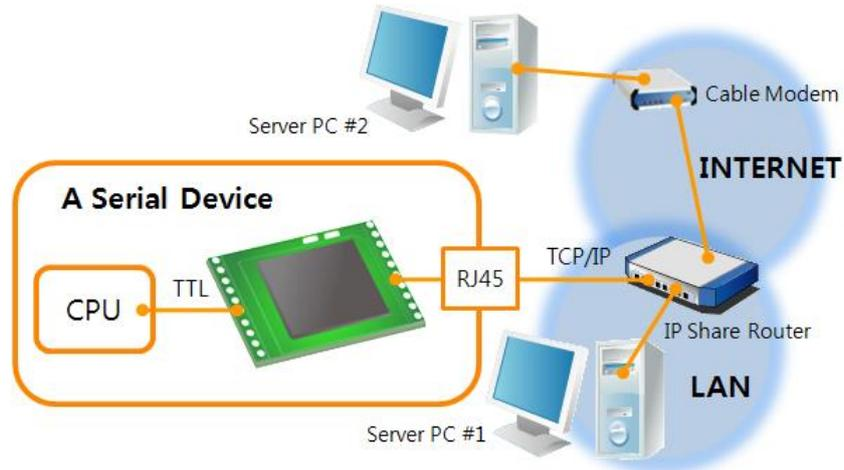
Figure 1-4 applied to the Internet with an IP share router
