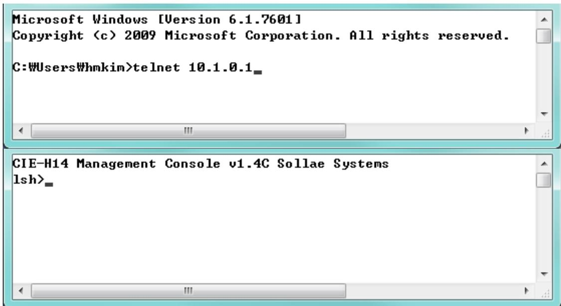
Figure 7-6 log in to CIE-H14 on TELNET
