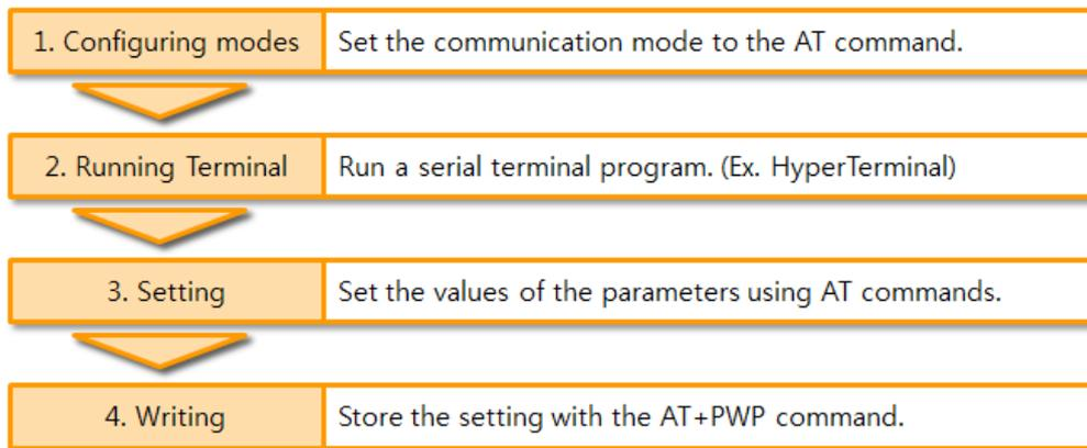
Figure 3-6 procedures for configuration with AT command
