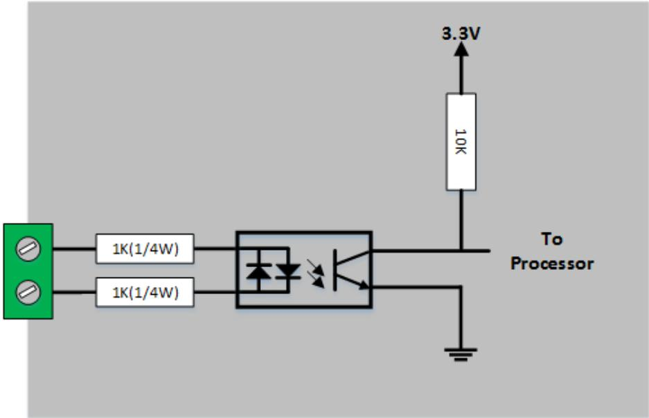
Figure 1-8 a circuit of the input port
