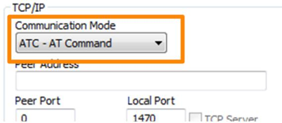
Figure 3-5 setting the communication mode to the AT command
