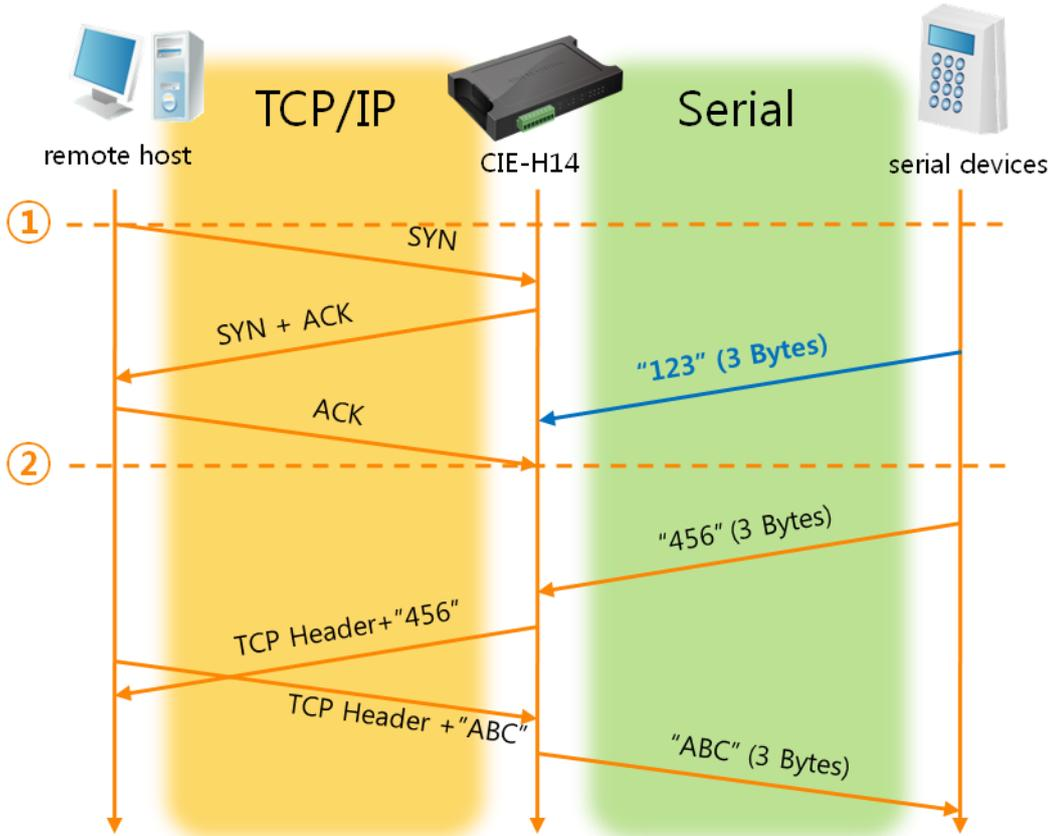
Figure 6-1 TCP server in the case [Event Byte] is set to 0
