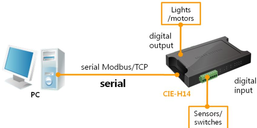
Figure 1-2 serialized Modbus/TCP
