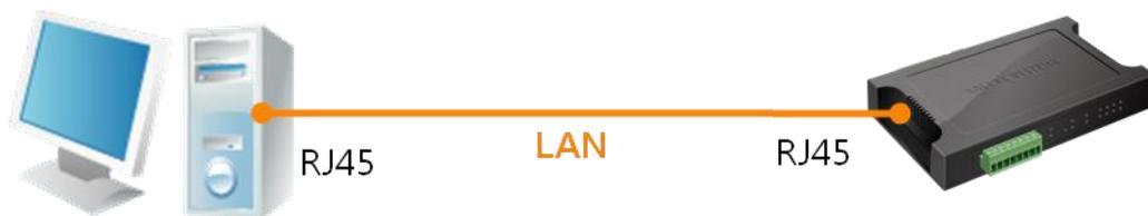
Figure 2-1 the connection between CIE-H14 and a PC
