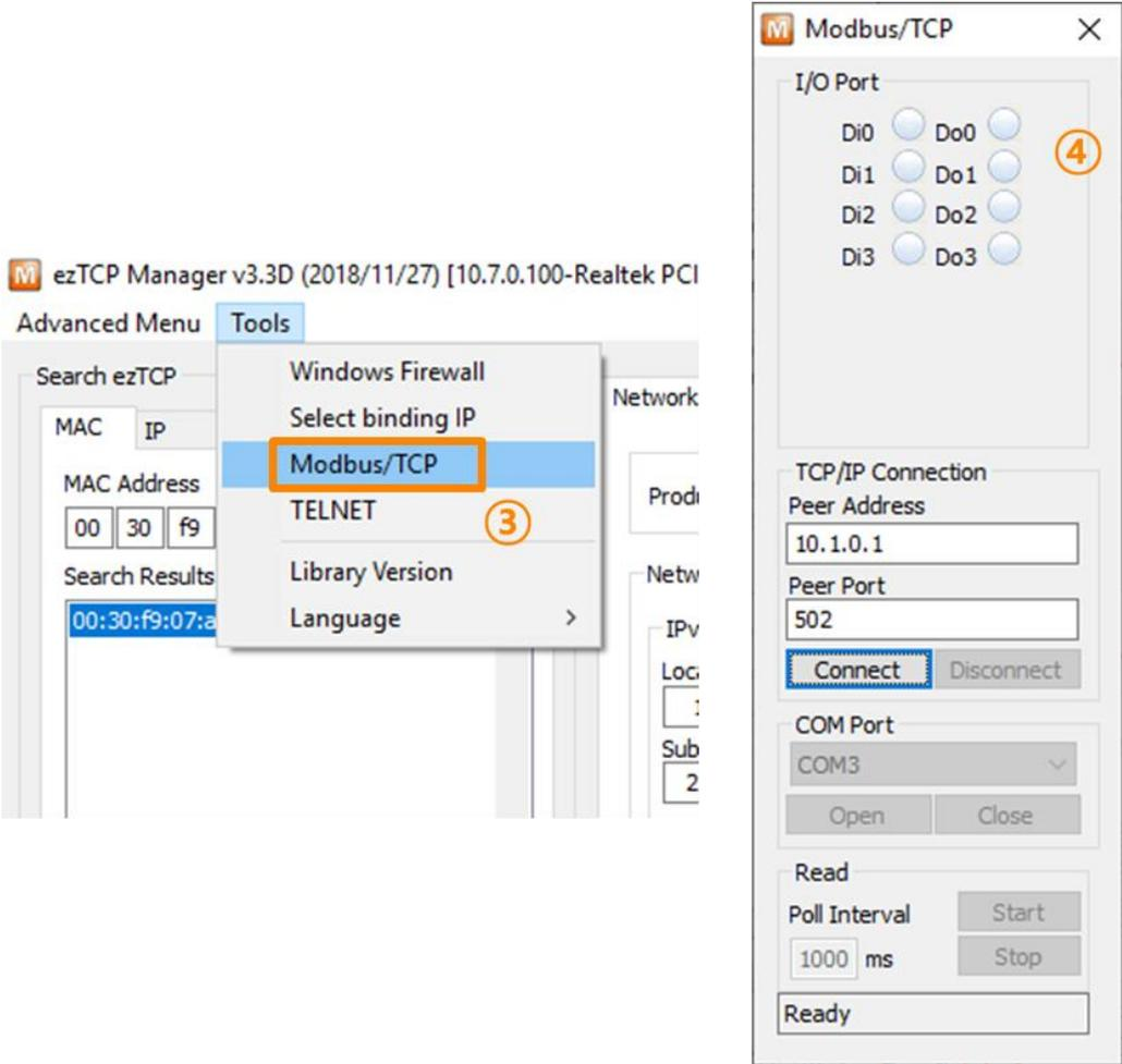
Figure 2-3 Modbus/TCP test program of the ezManager
