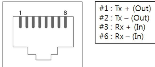
Figure 1-12 the RJ45 connector
