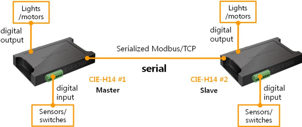
Figure 1-4 serial switch
