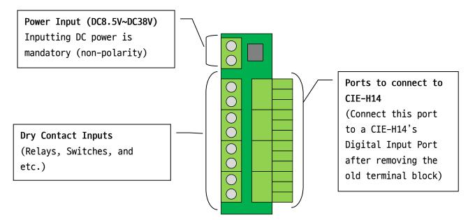
• An example : each contact input has two signal lines
