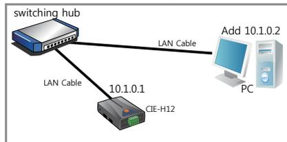
Connection map for configuration and the communication test
