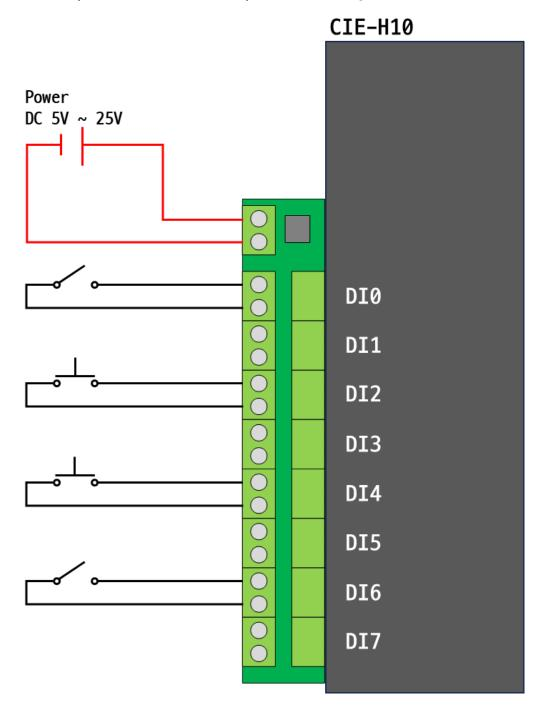
An example : contact inputs are composed of signal lines and a common line
