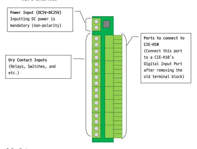
An example : each contact input has two signal lines
