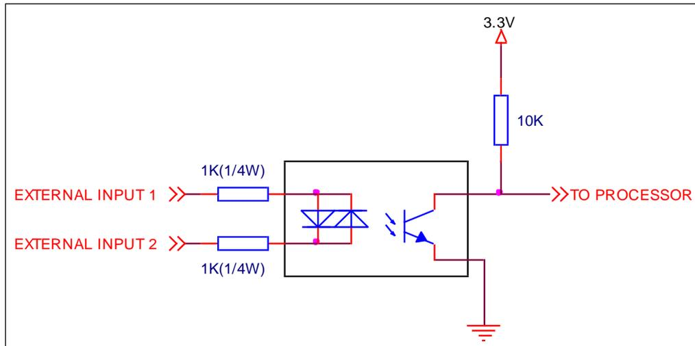
Figure 3-1 circuit diagram of an input port of CIE-H10
