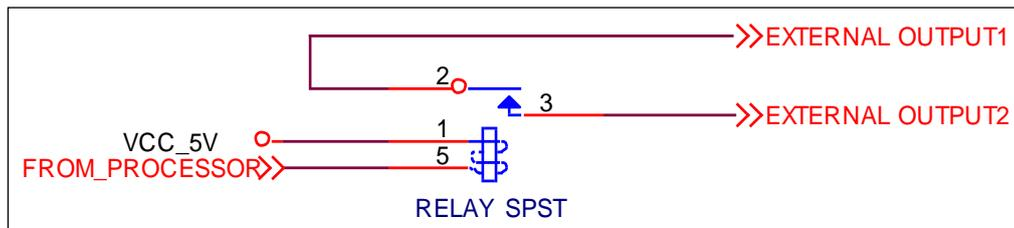
Figure 3-2 circuit diagram of an output port of CIE-H10
