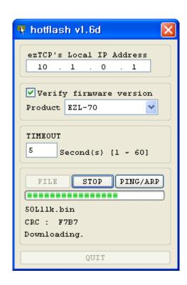
After completion, a message that informs the firmware was downloaded successfully. And EZL-70 reboots automatically and run in Normal Mode. In Normal Mode, the yellow LED is blinked every 1 second.
