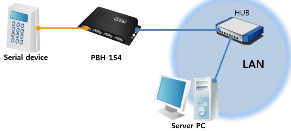
Figure 1-3 applied to LAN
